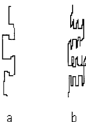
Figure 4 Orientational scheme of the PMMA chains in the elongated films: (a) long-range orientation; (b) short-range orientation and chain folding.
